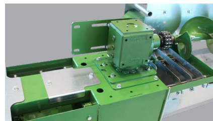
Center Sump with openings on both sides of the gearbox
